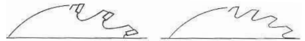
FIG 4. All rip saw blades are designed for fast, deep cutting. The harsh tearing action of a steel rip blade makes it generally unsuitable for any sawing operation other than timber ripping, whereas the cutting action of the TCT equivalent makes it suitable for general conversion duties in a wide variety of materials
